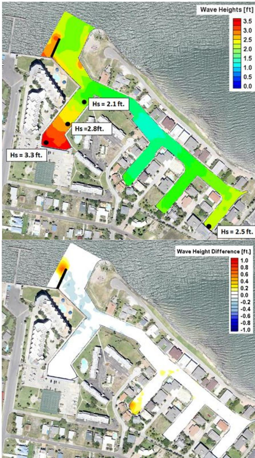
Figure A2. Maximum surge wave height (top) and surge wave height difference from existing (bottom) for Alternative 2.
