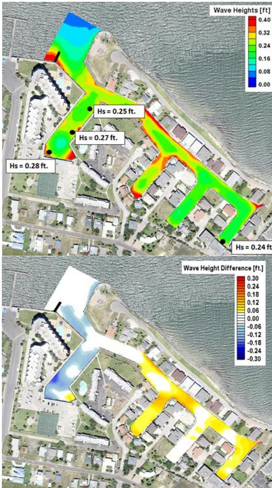
**Figure B5. Significant breaking wave height (top) and significant breaking wave height difference from existing (bottom) for Alternative 4.**
