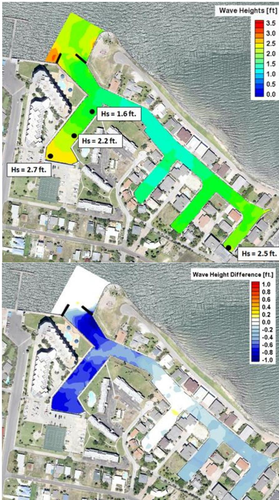
Figure A4. Maximum surge wave height (top) and surge wave height difference from existing (bottom) for Alternative 3A.
