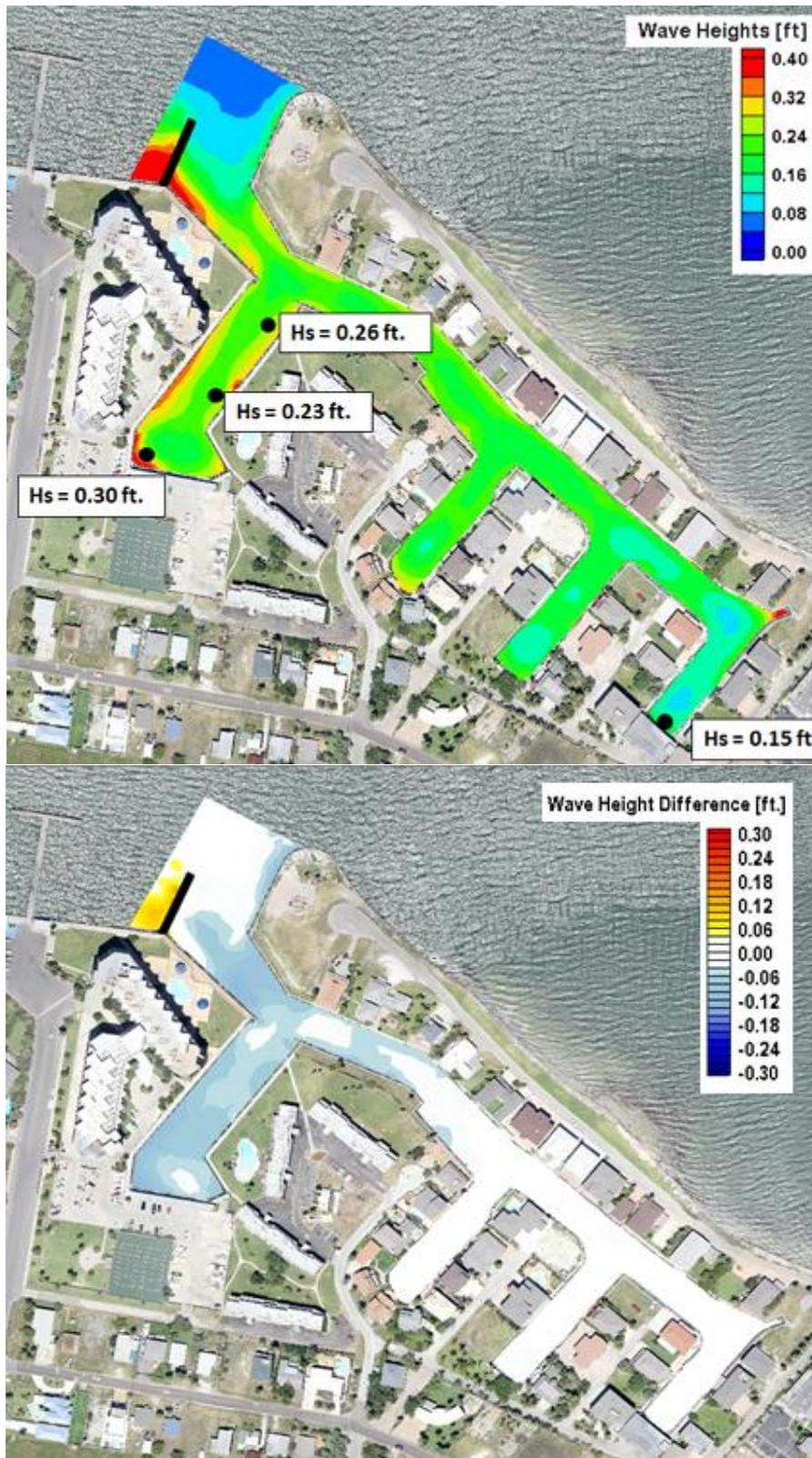
**Figure B2. Significant breaking wave height (top) and significant breaking wave height difference from existing (bottom) for Alternative 2.**
