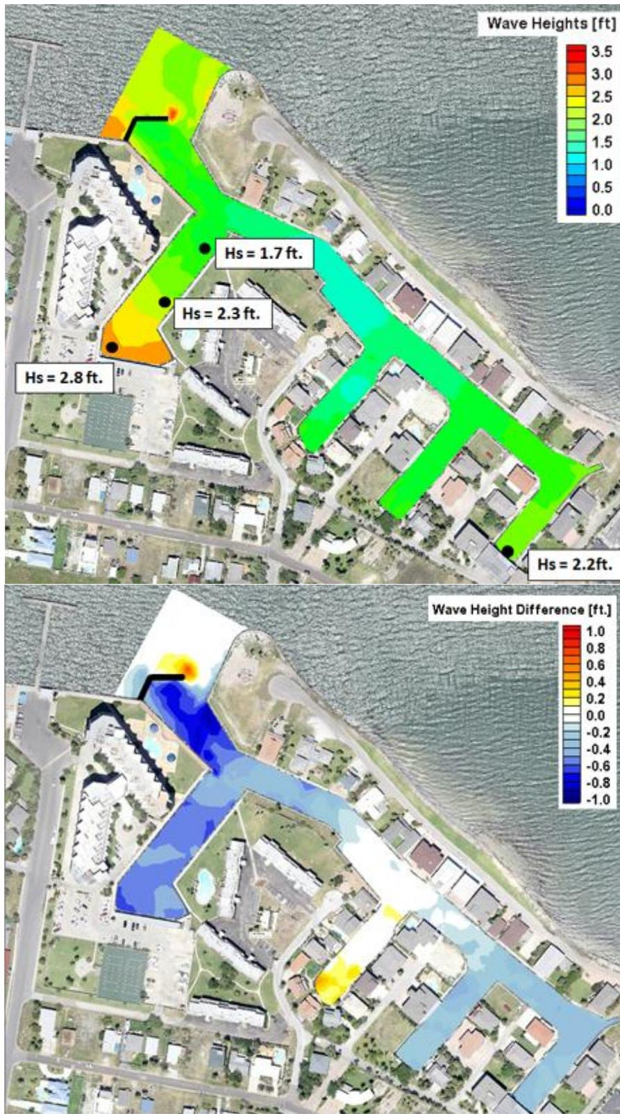
Figure A3. Maximum surge wave height (top) and surge wave height difference from existing (bottom) for Alternative 3.
