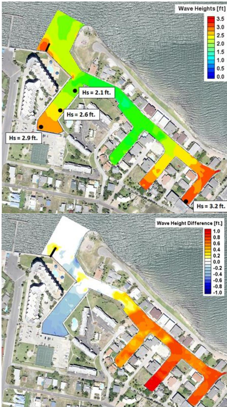
Figure A5. Maximum surge wave height (top) and surge wave height difference from existing (bottom) for Alternative 4.
