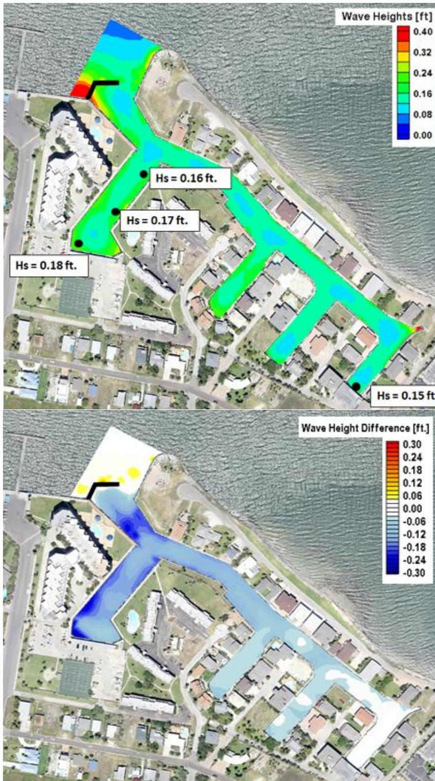
Figure B3. Significant breaking wave height (top) and significant breaking wave height difference from existing (bottom) for Alternative 3.
