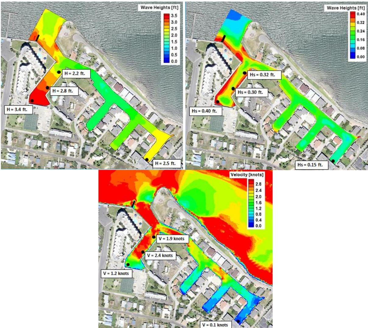
**Figure 7. Spatial plots for long period surge waves (top-left), short period breaking waves (top-right) and maximum velocity (bottom) for existing conditions (Alternative 0) with passing vessel at a speed of 10 knots.**
