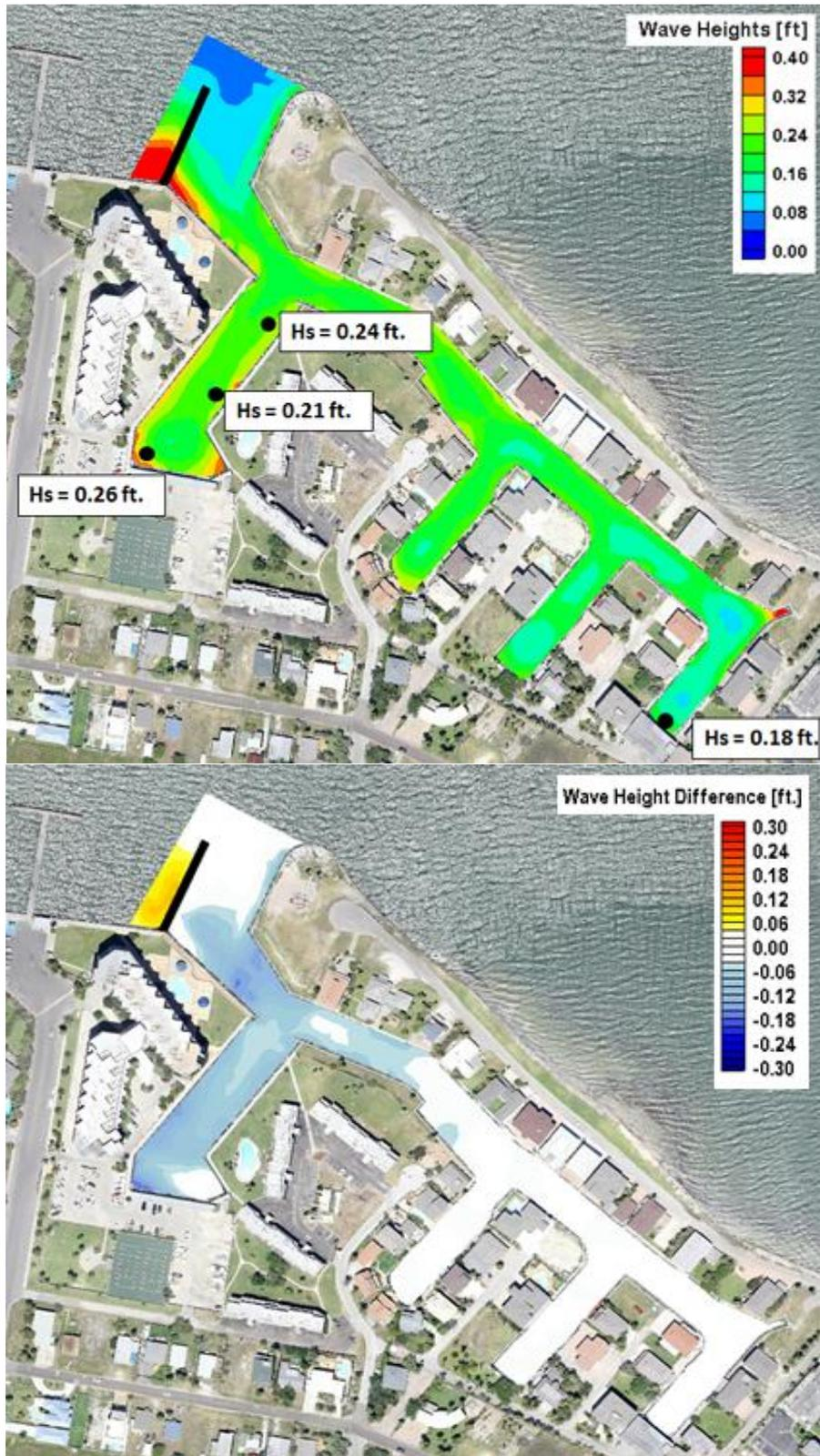
Figure B1. Significant breaking wave height (top) and significant breaking wave height difference from existing (bottom) for Alternative 1.
