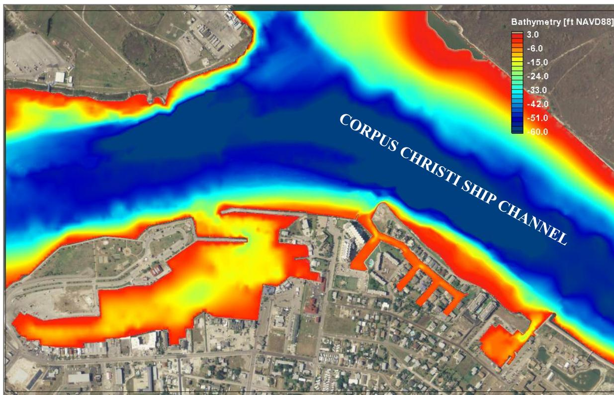
Figure 3. Bathymetry contours for the VH-LU modeling grid for existing conditions.
