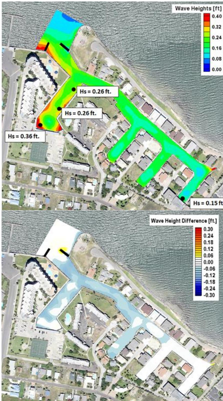
Figure B4. Significant breaking wave height (top) and significant breaking wave height difference from existing (bottom) for Alternative 3A.
