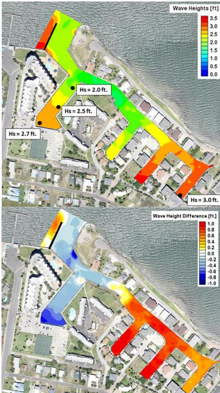
Figure A6. Maximum surge wave height (top) and surge wave height difference from existing (bottom) for Alternative 5.
