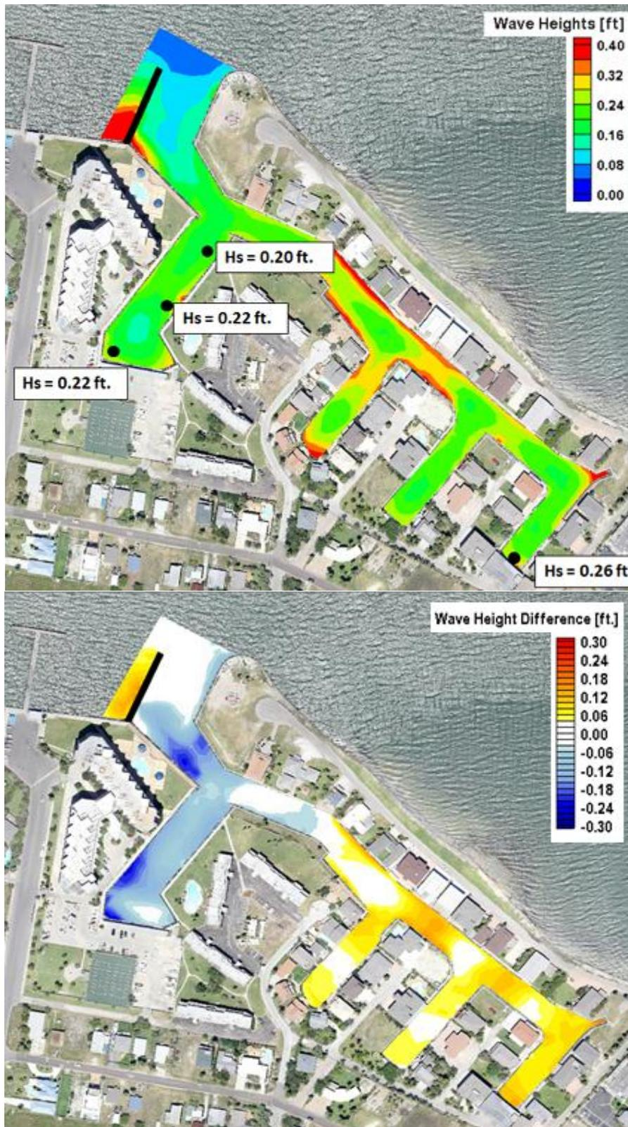
**Figure B6. Significant breaking wave height (top) and significant breaking wave height difference from existing (bottom) for Alternative 5.**
