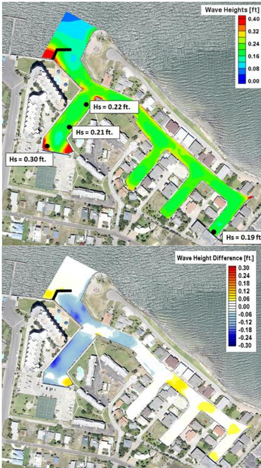
**Figure B7. Significant breaking wave height (top) and significant breaking wave height difference from existing (bottom) for Alternative 6.**
