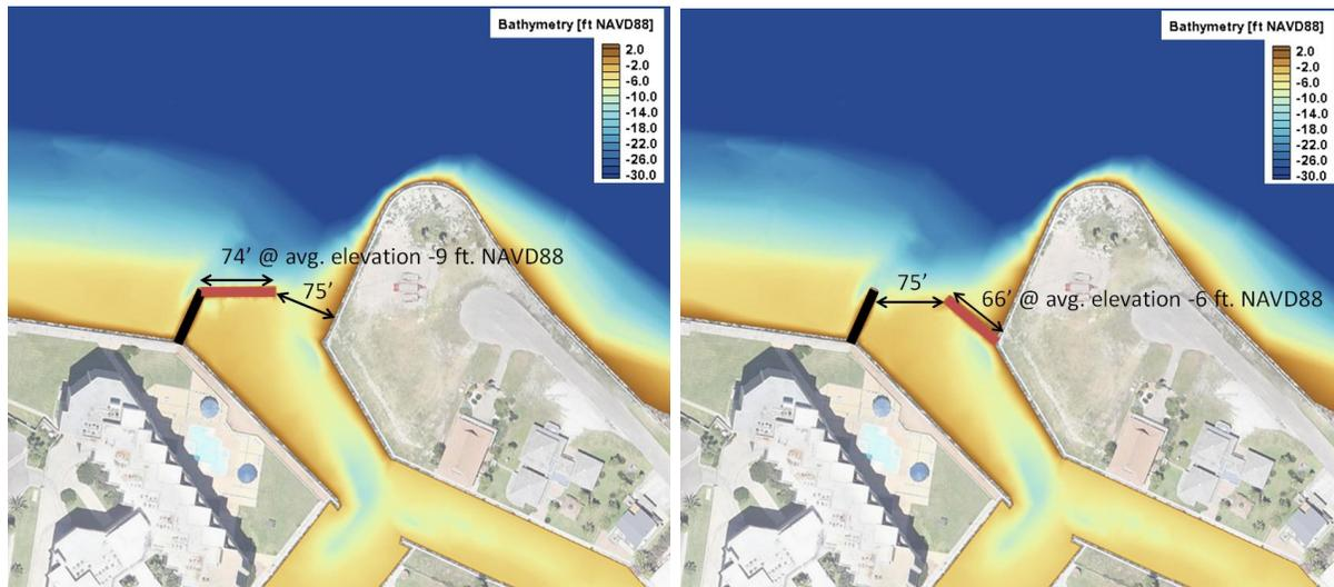
**Figure 9. Conceptual representation of Alternatives 3 and 3A.**
