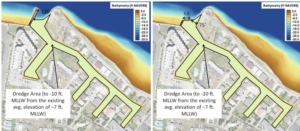
**Figure 11. Conceptual representation of Alternatives 5 and 6.**
