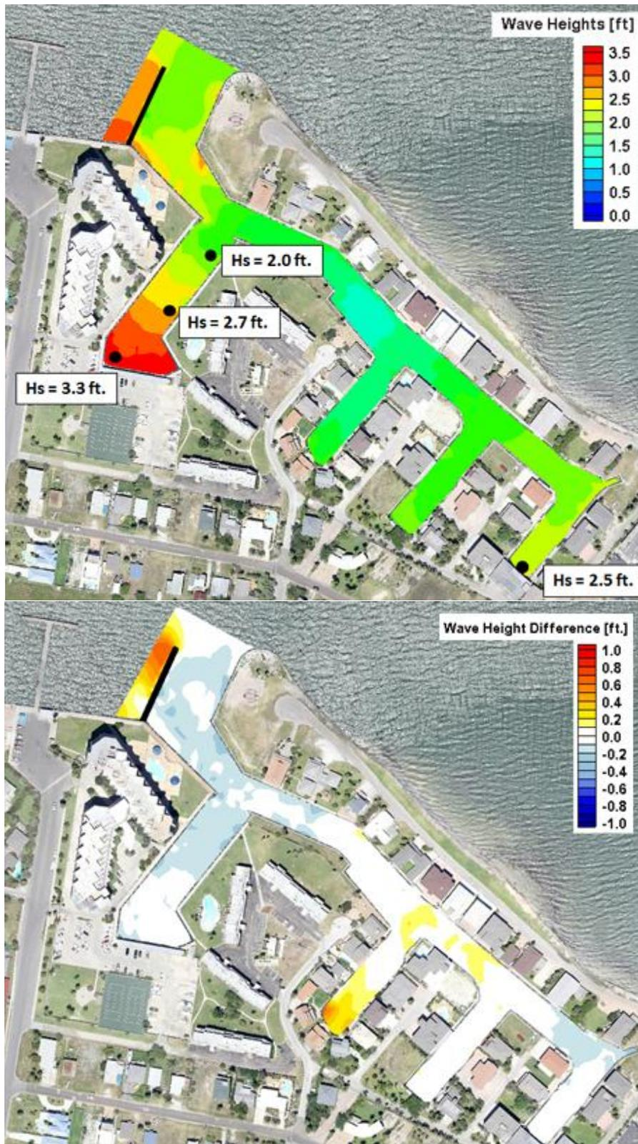
Figure A1. Maximum surge wave height (top) and surge wave height difference from existing (bottom) for Alternative 1.
