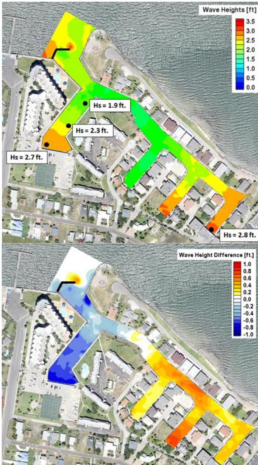
Figure A7. Maximum surge wave height (top) and surge wave height difference from existing (bottom) for Alternative 6.
