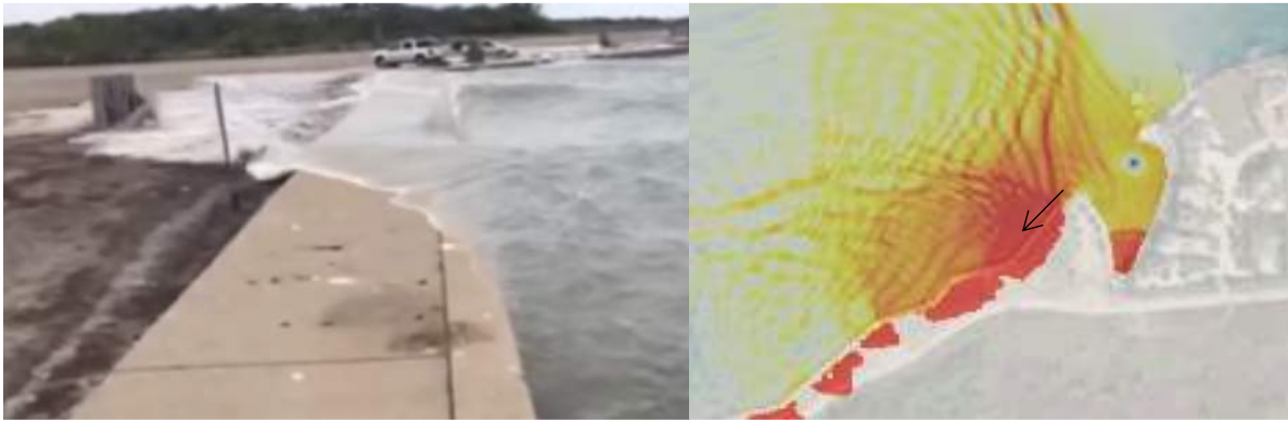
Figure 8. Comparison of overtopping extents for outbound case between observed (left) and modeled (right). Note: Arrow shows the approximate location and view point of the observed conditions.
