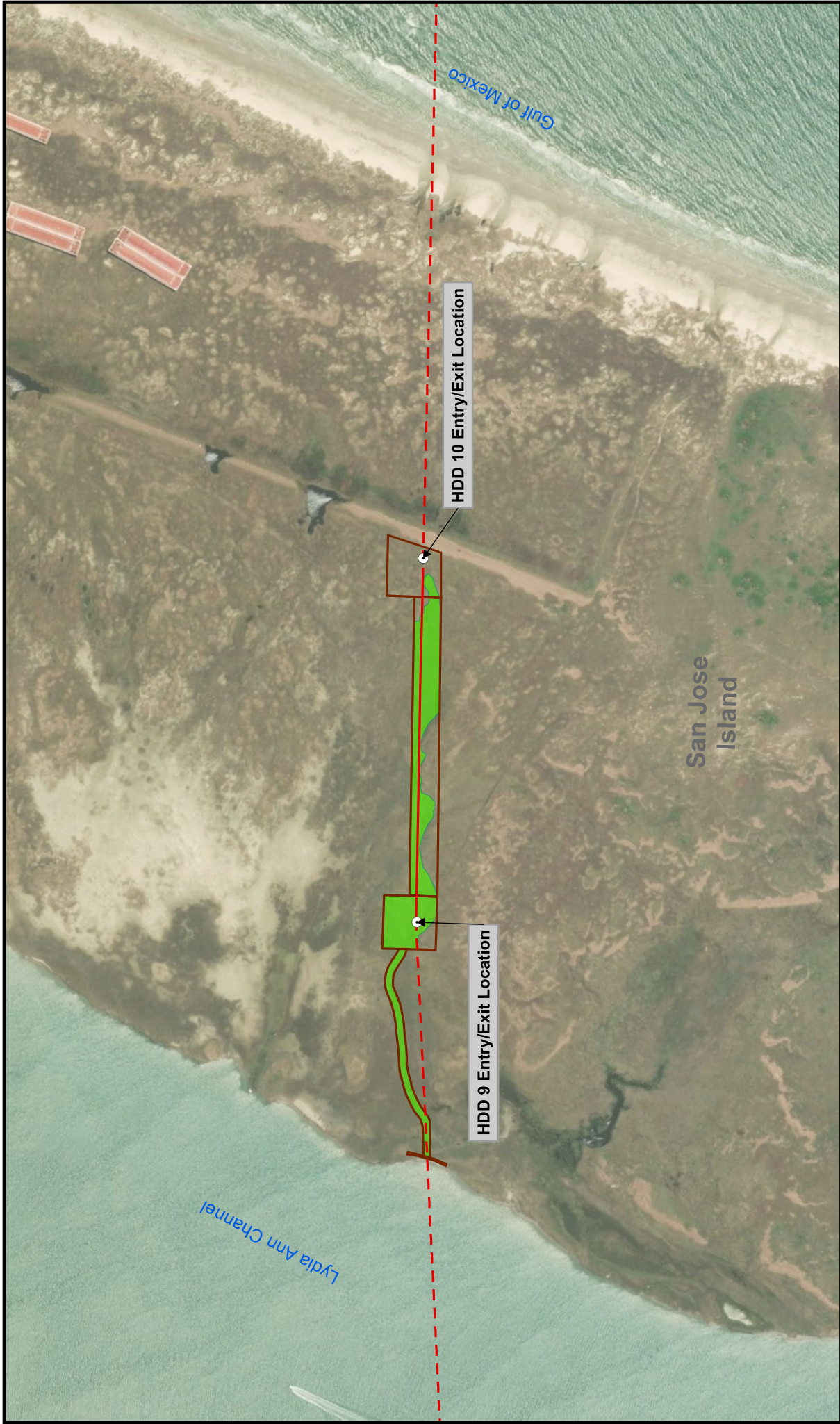
Figure 32 Proposed Project Detail Map Construction, Operation, and Decommissioning Procedures Bluewater SPM Project Bluewater Texas Terminal LLC
