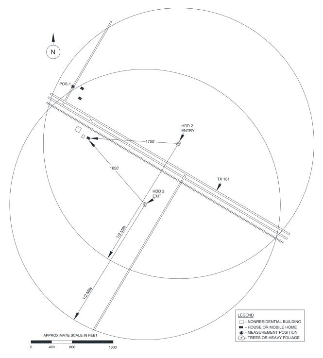
Figure 1:Bluewater SPM Project [HDD #2 (Highway 181 Crossing)]: Area Layout showing the<br/>HDD Crossing, HDD Entry/Exit Location and the Closest NSA(s).
