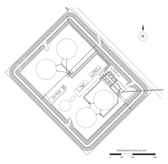
Figure 2:Bluewater Project Booster Station for Bluewater SPM Project: Drawing showing a<br/>Conceptual Layout (Plot Plan) of the Booster Station.
