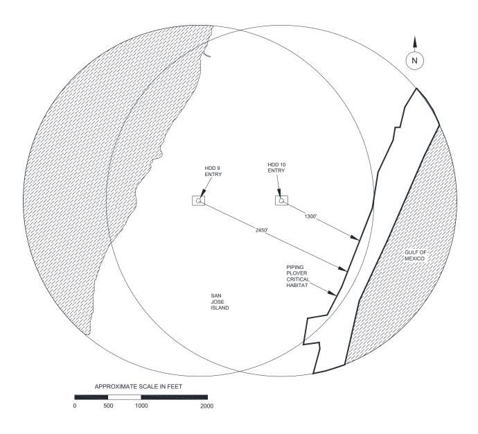
Figure 5:Bluewater SPM Project [HDD #9 and HDD #10 Entry Site (Inner Basin Waterway<br/>Crossing and Pipeline Installation to SPM)]: Area Layout showing the HDD Crossing(s),<br/>HDD Entry Locations and the Closest NSA (consisting of Piping Plover Critical Habitat).
