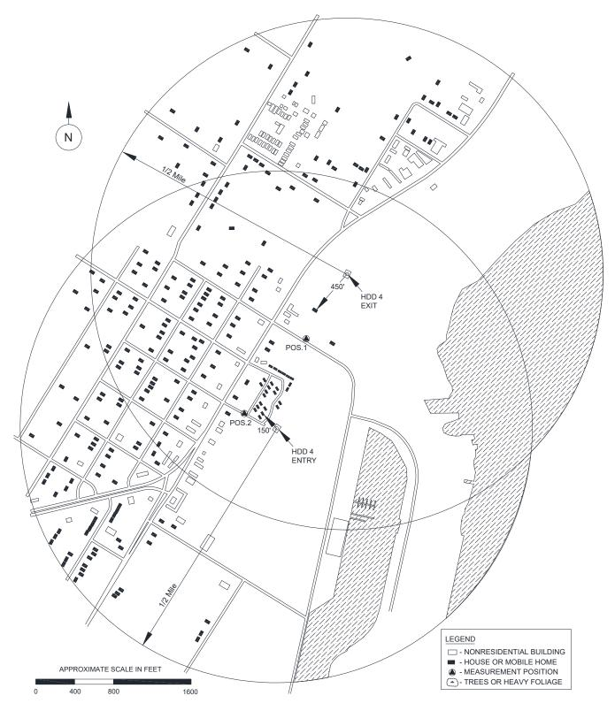
Figure 2:Bluewater SPM Project [HDD #4 (Crossing of E. Stapp Ave. & Water Bodies)]: AreaLayout showing the HDD Crossing, HDD Entry/Exit Location and the Closest NSA(s).
