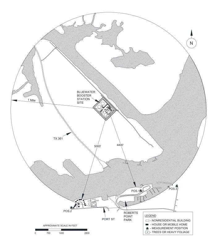
Figure 1:Bluewater Project Booster Station for Bluewater SPM Project: Area Layout/Map showing<br/>the Planned Site of Booster Station, NSAs within approximately 1 Mile of the Booster<br/>Station Site and Chosen Sound Measurement Positions near the Closest NSAs.
