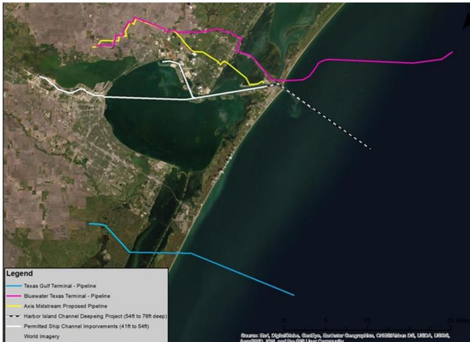
Figure 12. Map showing proposed 78-foot deep water channel into Harbor Island by dotted line and the 50-foot deep Corpus Christi Ship Channel in white. Also shown are the Texas Gulf Terminals offshore monobuoy in blue and the Bluewater Texas Terminal monobuoy in pink. Image by Sustainable Planning and Design.
