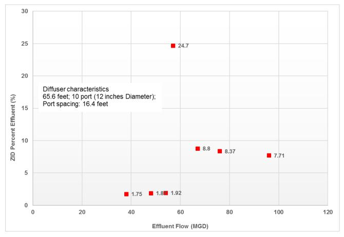
Figure 5: Discharge Flow vs. ZID Percent Effluent for the Specified Diffuser Design Alternative
