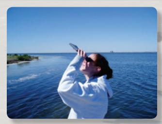
Measuring salinity using a refractometer.
