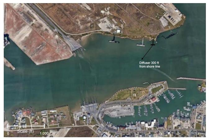
Figure 4: Proposed Location for Harbor Island Facility Diffuser
