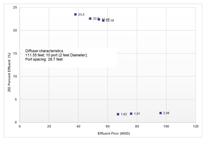
**Figure 6:** ZID Percent Effluent vs. Effluent Discharge Rate for the Specified Design Alternative at 40% RO Recovery
