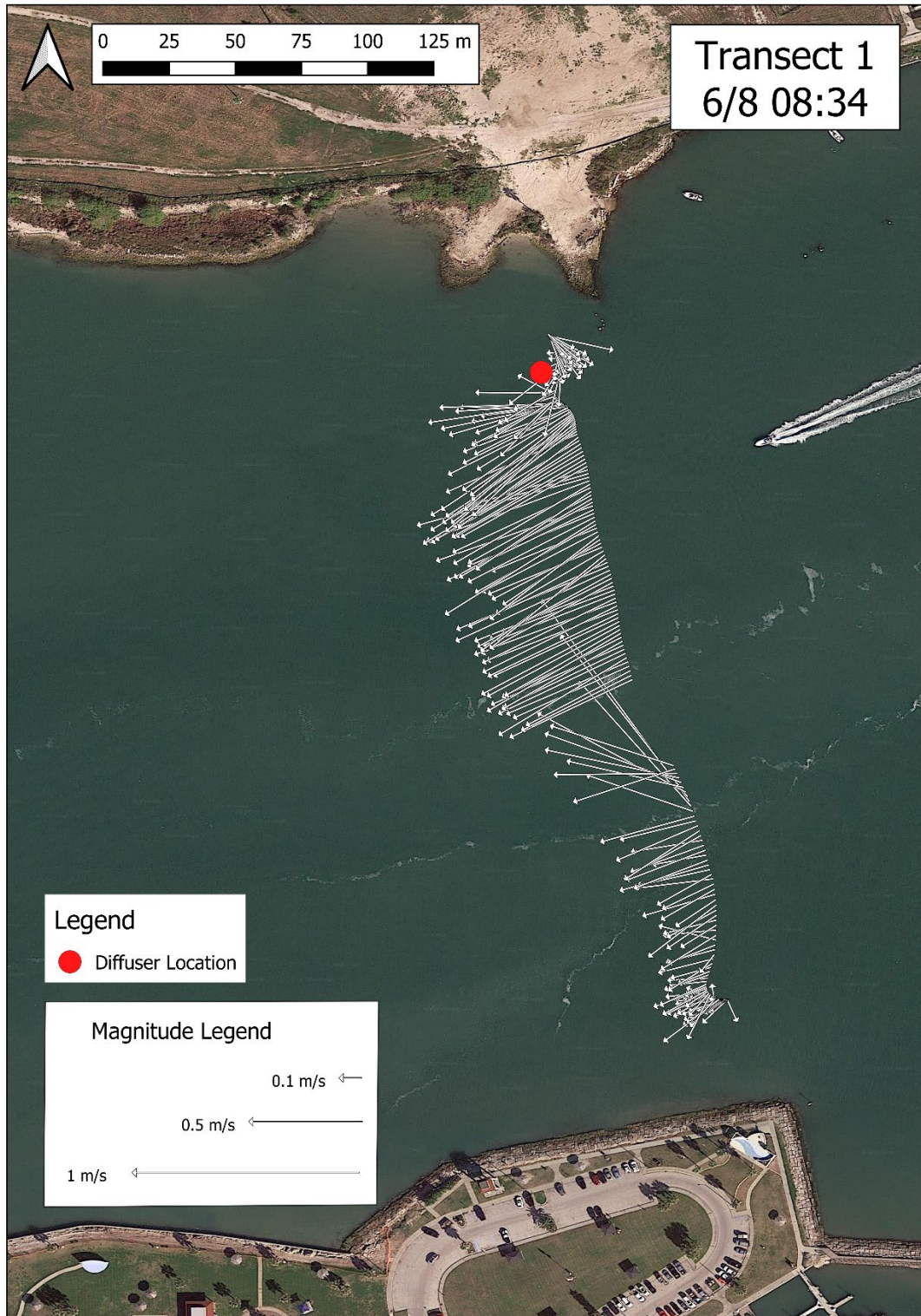
2 Figure 3. Depth-averaged velocity vectors from ADCP transect T1 starting on June 8 at 3 8:34am, with data averaged in the horizontal at one per second (approximately two 4 ensembles).
