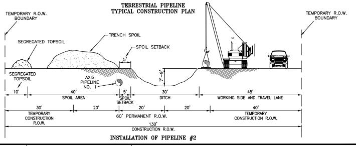
NOTE: THE CONTENT OF THIS DRAWING IS DESIGNED SPECIFICALLY FOR THE PURPOSE OF SECURING FEDERAL, STATE AND LOCAL ENVIRONMENTAL/ REGULATORY AUTHORIZATIONS ONLY.
