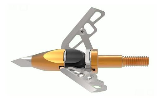
The broadhead blades are closed at impact, but open fully to their 1.65" diameter cutting radius and create an entrance wound.
