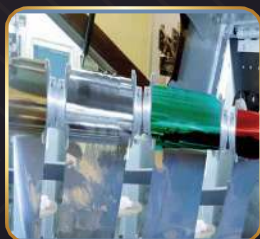
Utilize multiple foil rolls simultaneously, with a maximum of 4 rolls each with a width of 4 inches.
