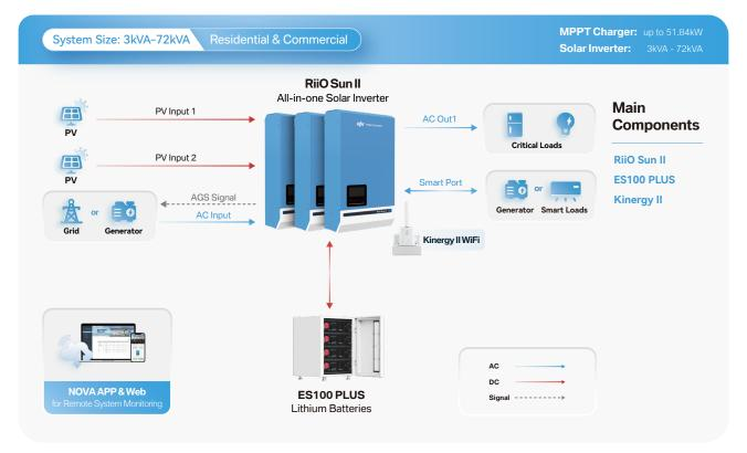
With its transformer-based design, AGS, Power Assist and Power Control functions, RiiO Sun II ensures stable operation of critical loads during power interruptions or in pure off-grid scenarios. Built-in with 2 MPPTs and a programmable smart port, the solution offers greater flexibility for system design based on users needs and enables intelligent energy management.
