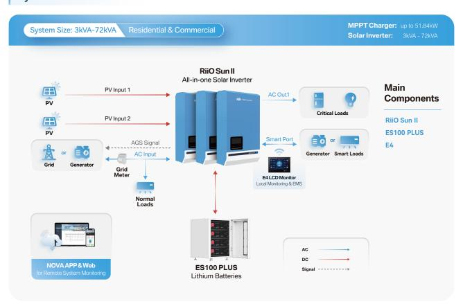
Ideal for regions with a reliable grid but high electricity costs. RiiO Sun II supports feeding energy back to power loads on the AC input to to maximize solar self-consumption. With TBB E4 LCD Monitor, the solution can further reduce your electricity bills with peak shaving and time-of-use strategies.
