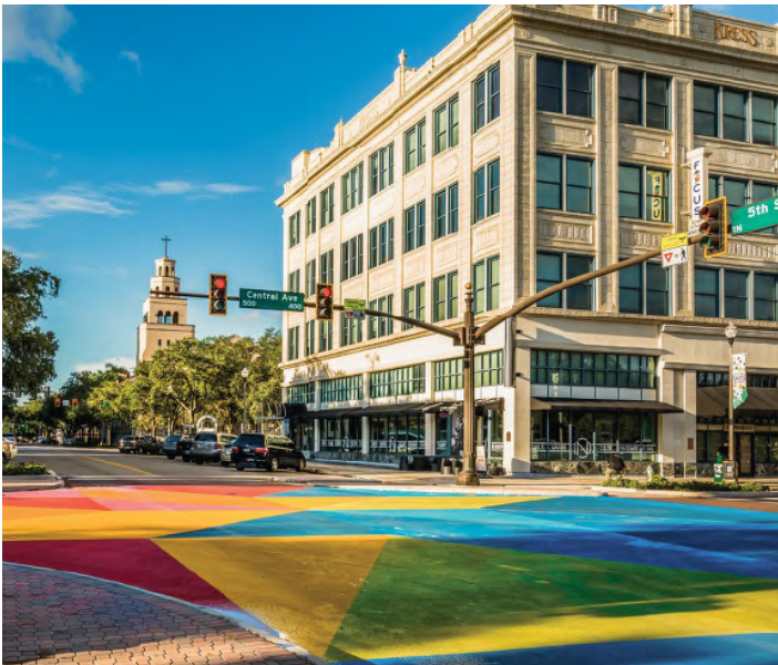
Painted Intersection for Traffic Calming (Asphalt Art Guide)
