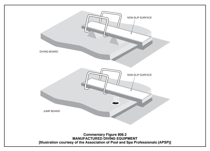
**808.9 Location.** The forward tip of manufactured or fabricated diving equipment shall be located directly above Point A as defined by Section 808.6.
