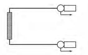
Figure 5. Single unblockable channel outlet to two pumps.
