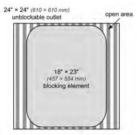
Figure 3a. Example of unblockable suction outlet
