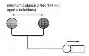
Figure 9. Dual outlets in parallel to one pump
