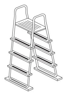
FIGURE 702.2 TYPICAL A-FRAME LADDER, TYPES A AND B
