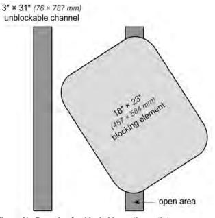
Figure 3b. Example of unblockable suction outlet
