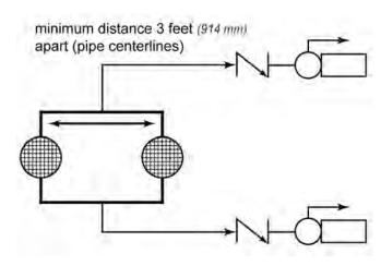
Figure 11. Dual parallel outlets to two pumps
