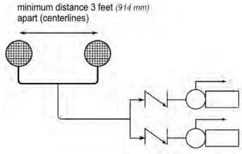
Figure 10. Dual outlets in parallel to dual pumps
