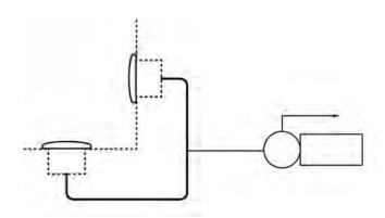
Figure 12. Dual outlets on different planes
