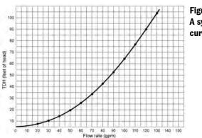
Figure 2. A system curve
