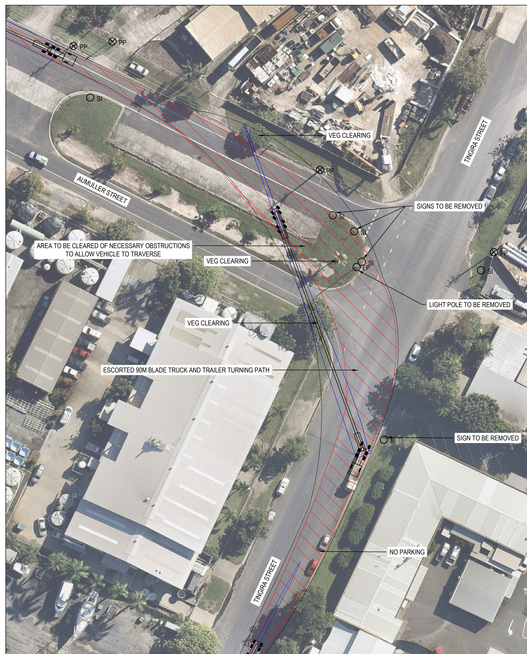
AUMULLER STREET / TINGIRA STREET INTERSECTION - 90m BLADE TRUCK AND TRAILER (TRAVELLING TO LAYDOWN)
