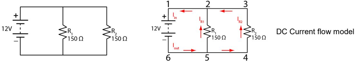
We know the voltage drop across each resistor in each branch of this parallel circuit is 12V.
