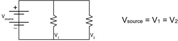
In other words, if the source voltage is 12 Volts each branch circuit will conduct the full 12 volts.
