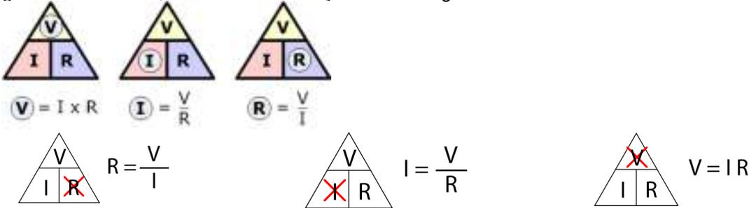
For example, to find resistance (R) when given the voltage (V) and the current (I), cover the "R" and you'll get the formula for resistance  $R = V/I$ .
