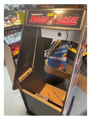
3. Install the Gen 1 monitor and PCB (exact same size as the one that came out of the cabinet, also same screw pattern). Then install the new j panel, after this tighten all of the side screws
