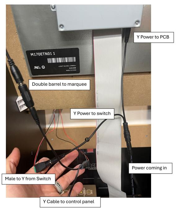
5. Connect power from Y cable to LED cable on control panel, then connect PCB ribbon cable
