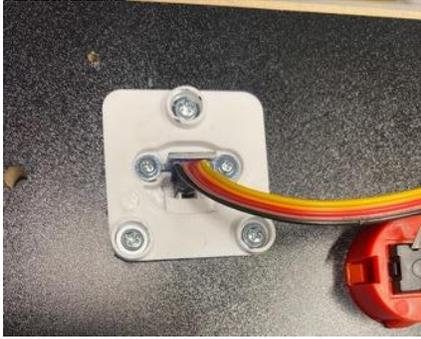
Step 7- Lightly pry up the headphone jack surround with a small flat head screwdriver
