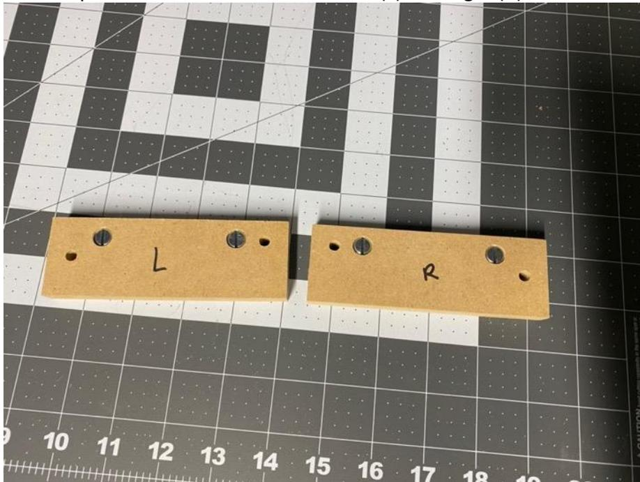
Install the Cross Barrel Insets into the deck with the Flathead screw slot facing vertical
