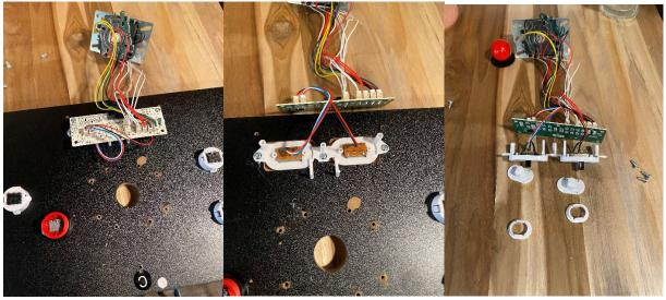
Step 5- Remove encoder board, encoder board support, VOL/PWR buttons, and surrounds
