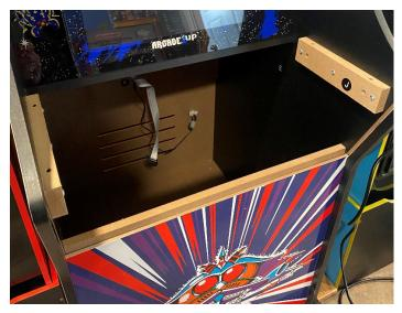
Step 2- Remove rear black plastic cover (This will not be reused and can be discarded, recycled, store in the base of the cabinet).
