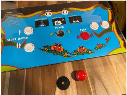
Step 3- Remove the Ball and Dust Cover
