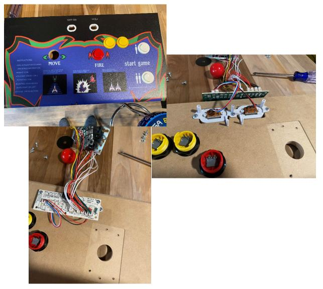
Step 7- Reinstall Joystick and connect buttons
