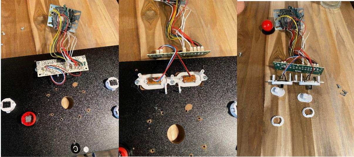
Step 6- Install surrounds in new deck and reinstall encoder board support and board
