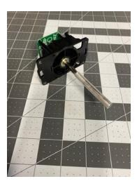
Step 10- Install LED Holders into Front Plate, making sure to install on correct side (opposite side from first image). May need to VERY LIGHTLY sand the corners as it is a snug fit (image 2). Final image shows installed correct positions.
