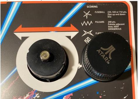
Step Two- Remove cable from spinner and remove spinner, some light prying on the edges of the spinner should remove it.
