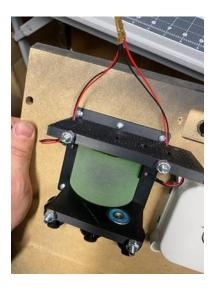
Step 13- Reinstall Power/ Volume/ PCB Holder and install standoff
