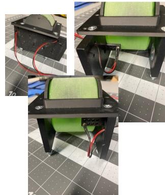
Step 12- Use the 6 Pan Head Screws provided to secure the controller (DO NOT OVERTIGHTEN slowly screw to just snug otherwise will show through front) Front plate should face front towards screen.
