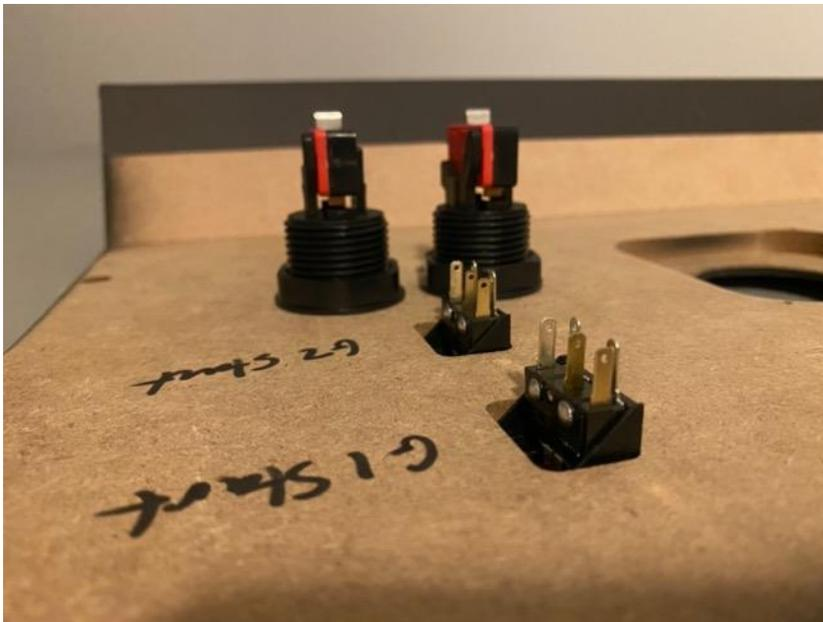
Step 16- Connect LED harness to Volcano LEDs and Green LEDs
