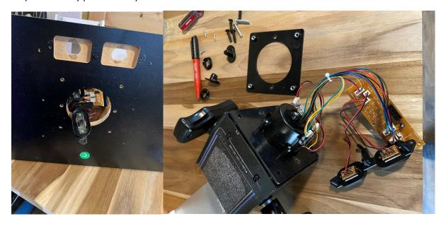
Step 7- Prepare replacement panel by install the surrounds and button sliders the carefully pull the encoder board and yoke through the panel, and install screw plate and the two silver screws (LEAVE THESE SCREWS A FEW TURNS LOOSE TILL THE VERY END TO MAKE INSTALL EASIER)
