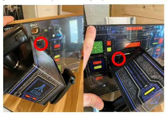
Step 5- Remove 2 silver screws from the back of the control panel and remove screw collar while removing the power and volume surrounds (use Goof Off and a Q Tip to dissolve any glue for easier removal)
