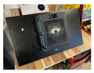
Step 3- Remove the encoder board and support (it is NOT necessary to remove any wiring).
