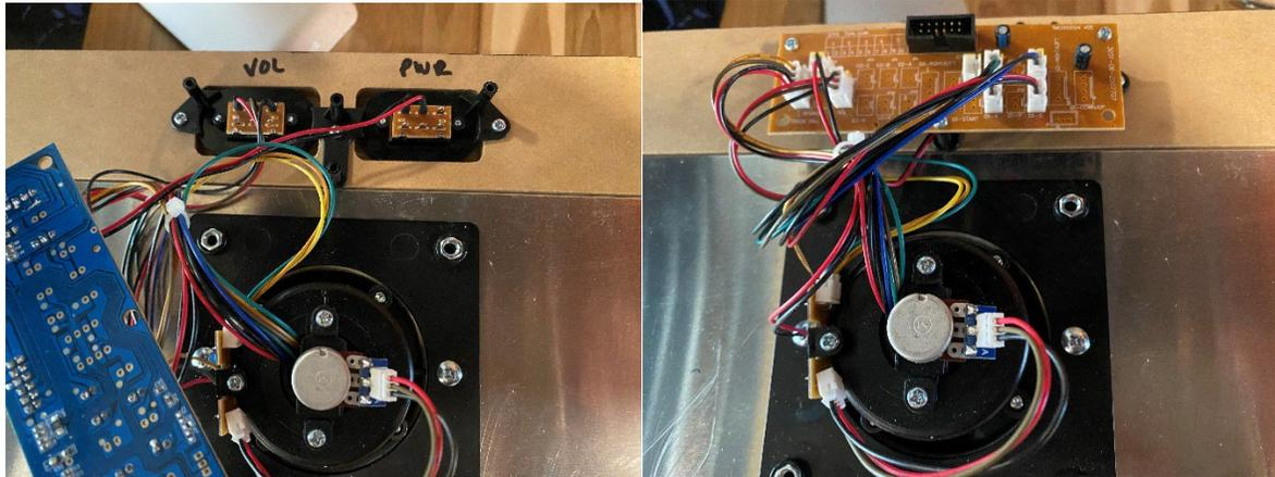
Step 9- Reinstall the 4 black screws through the front of the panel (this is the trickiest part of the install, leave all screws just loose until all 4 are seated and then tighten in a cross pattern, turn the deck over and final tighten the two silver screws)
