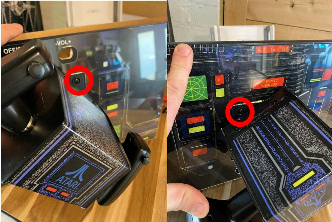
Step 5- Remove 2 silver screws from the back of the control panel and remove screw collar while removing the power and volume surrounds (use Goof Off and a Q Tip to dissolve any glue for easier removal)
