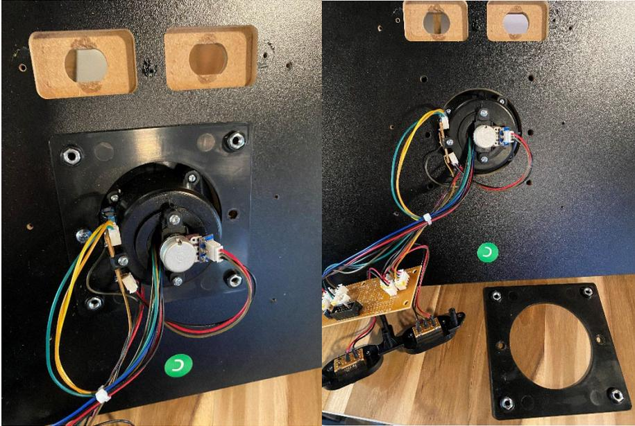
Step 6- Carefully pull out the yoke and the encoder board with the wires attached
