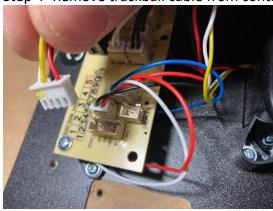
Step 5- Remove trackball from deck, when reinstalled cord must be facing north as indicated on the deck otherwise trackball orientation will be incorrect.
