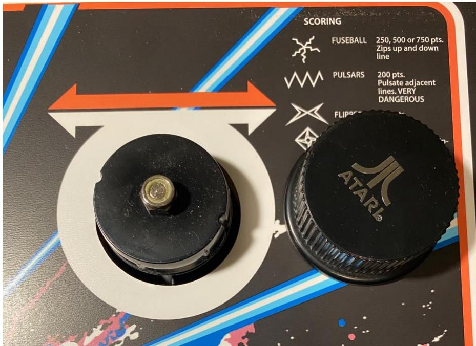
Step Two- Remove cable from spinner and remove spinner, some light prying on the edges of the spinner should remove it.
