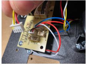
Step 5- Remove trackball from deck, when reinstalled cord must be facing north as indicated on the deck otherwise trackball orientation will be incorrect.
