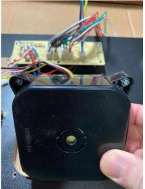
Step 6- Remove top screws from control board, then remove lower screws from VOL/ POWER mount.
