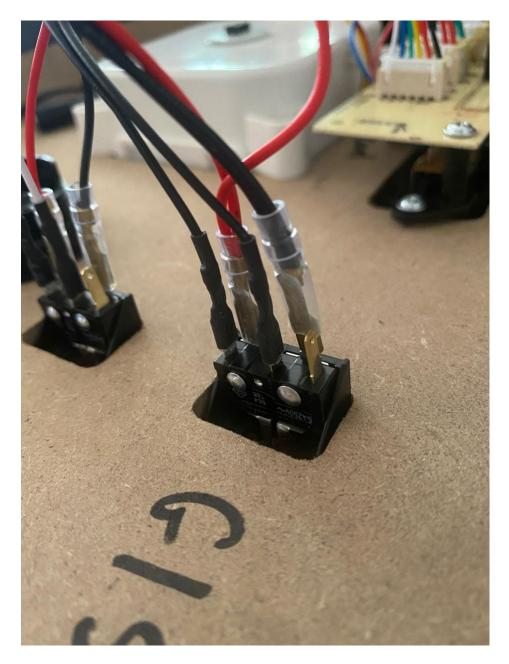
Step 9- Connect LED harness to Volcano LEDs
