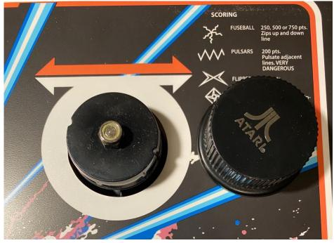
Step 1- Remove the spinner cap, a little bit of pressure to lift it will suffice.
