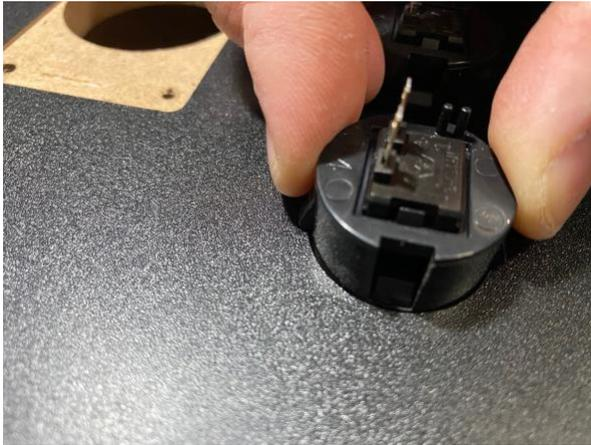
Step 4- Remove trackball cable from control board.
