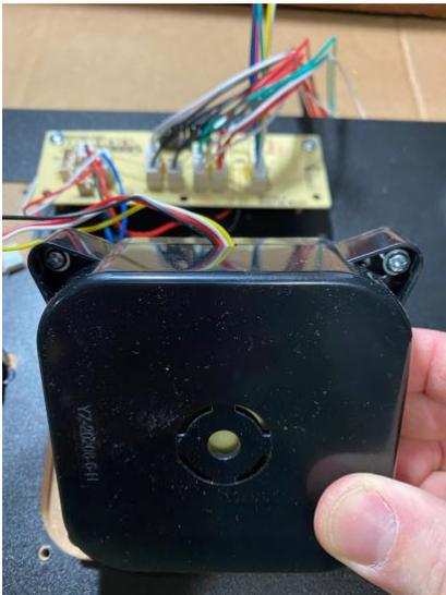
Step 6- Remove top screws from control board, then remove lower screws from VOL/ POWER mount.
