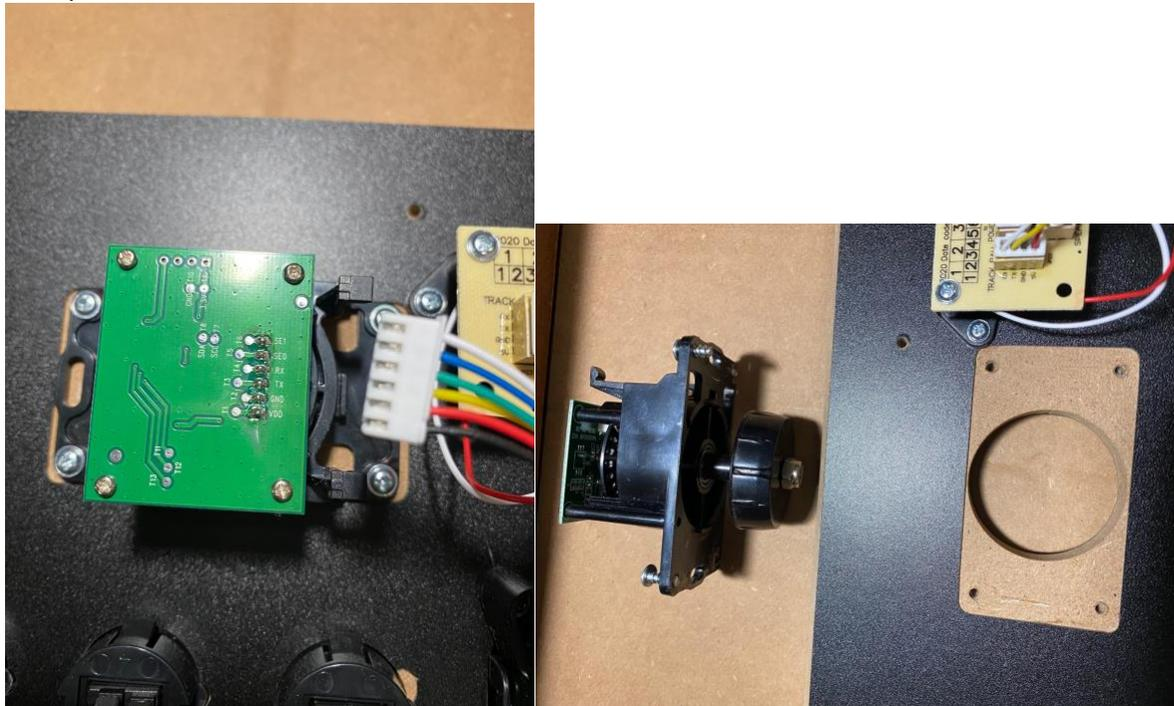
Step 3- Remove cables from buttons and pinch sides to remove, all button locations are already mapped on your deck so no need to label. Polarity on the cables does not matter, either side can be connected.
