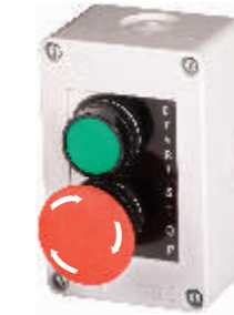
Flush Head Actuator - Green with Legend - START Contact - 1 'NO' (Station One) Mushroom Head Actuator 'Push Turn Type' with Legend - STOP Contact - 1 'NC' (Station Two) Cat. No. : JBB2F100
