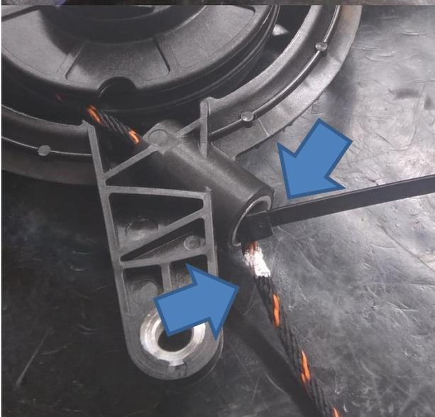
Insert the rope into the rope guide.
