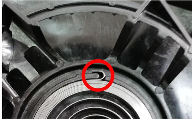
Insert the spring of the hooks on the central pin and turn it, if any blockage or jamming occurs the pin must be replaced.
