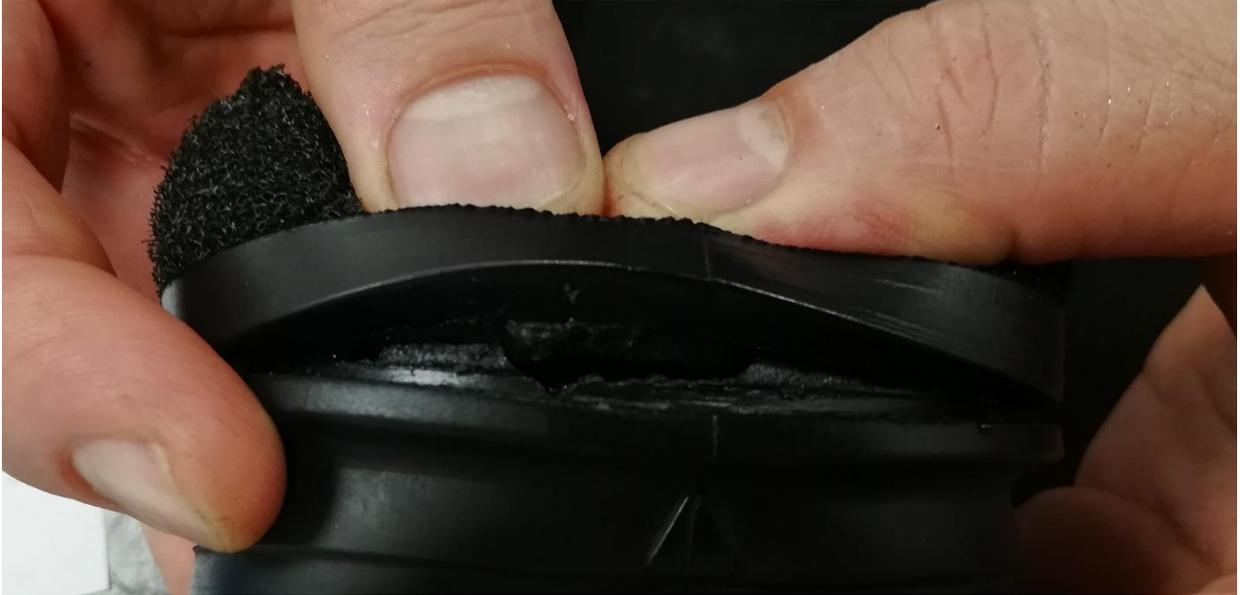
Check the filter, in particular the bonding with the sleeve and the various parts of the sponge.
