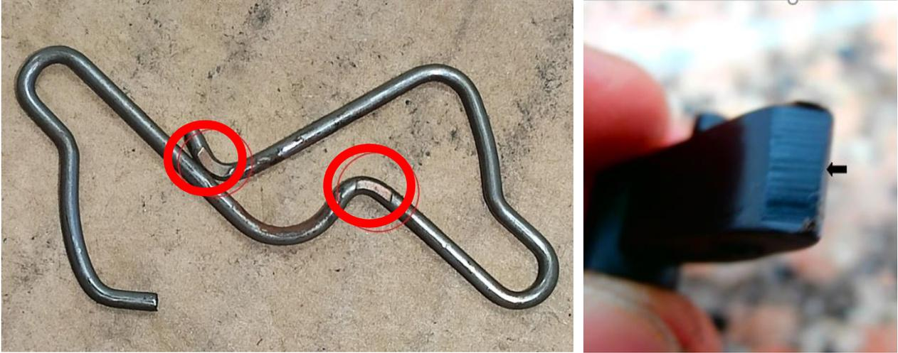
Check the hooks, in particular the tips must not be damaged, otherwise they must be replaced. For routine maintenance, follow the table.
