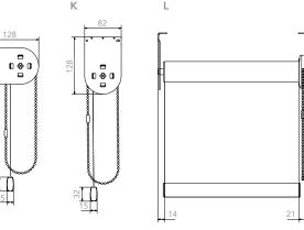
• J. System 45<sup>®</sup> Extended Metal Bracket Face Fix • K. System 45<sup>®</sup> Extended Metal Bracket Top Fix • L. System 45<sup>®</sup> Extended Metal Bracket Top Fix Front View
