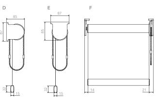
• D. System 45<sup>®</sup> with Enclosed Bracket Covers Face Fix • E. System 45<sup>®</sup> with Enclosed Bracket Covers Top Fix • F. System 45<sup>®</sup> with Enclosed Bracket Covers Top Fix Front View
