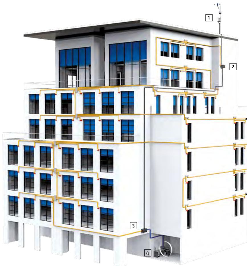
The animeo IP/RS485 Building Controllers and Sub Controllers are communicate bi-directionally with the motors.
