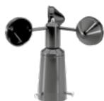
To measure wind speed in connection with the Outside Sensor Box.
