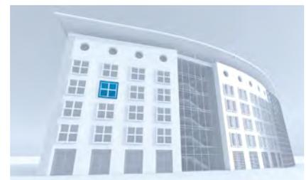
Within the same zone, all blinds behave the same way. Smaller zones enable more efficient and precise operation.
