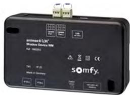
The LON Shadow Device stores the relevant data which is derived from building model provided through Somfy. It is essential in conjunction with the animeo LON Motor Controller to realize window based shadow tracking for buildings.
