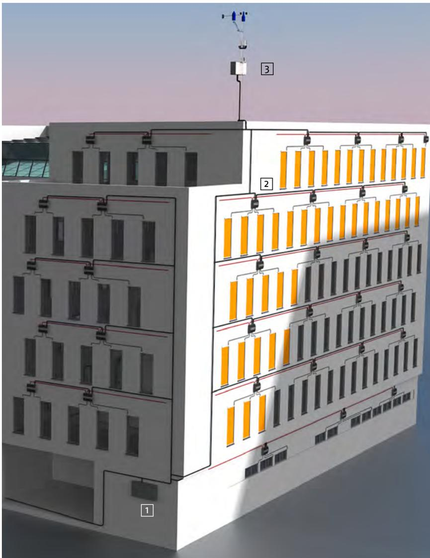
The LON network enables creation of any network topology for all LON products installed (Motor Controllers/ Sensor Station).
