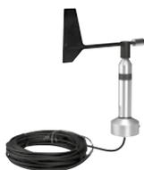
To measure wind direction in connection with the Outside Sensor Box.
