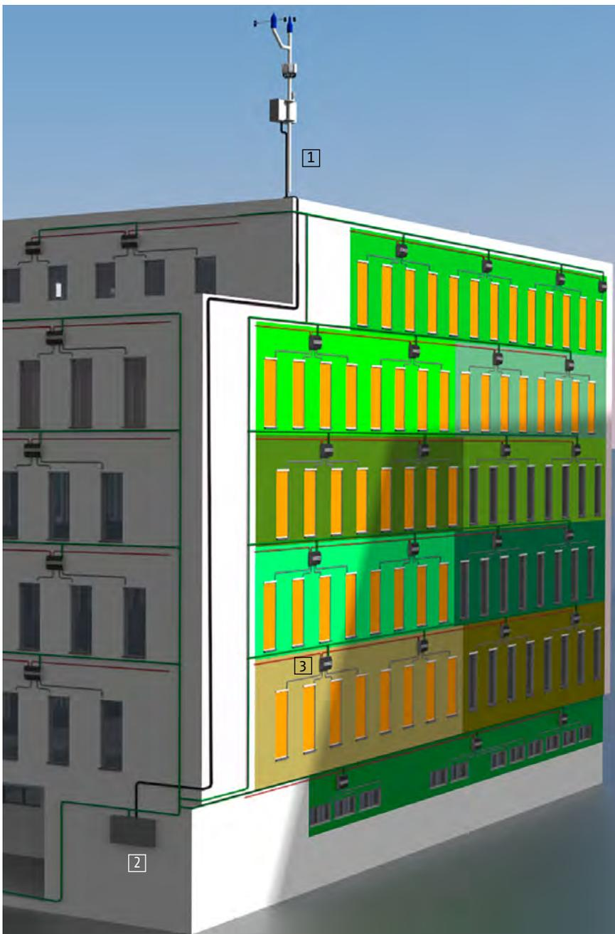
All the Motor Controllers are connected to the same KNX network via the animeo KNX Master Control.
