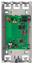
KNX RS485 Motor Controller enables the controlling of up to 18 motors. The motors can be controlled either individually or by groups.
