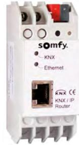
The KNX/IP router enables telegrams to be forwarded between different lines through a LAN (IP) as a fast backbone. In addition, this device is able to connect a PC to the KNX network e.g. for ETS programming. The IP address can be obtained by a DHCP server or by manual configuration (ETS) respectively.
