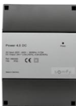
To supply power to the DC Motor Controller. In the application of "Somfy Concept 25" motors, up to 2 LON Motor Controller 4 DC can be supplied by one power supply (= 8 motors). Switchable also in parallel:  $2 \times 4.5 \text{ A} = 9 \text{ A}$ .
