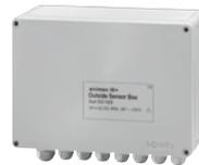
The Outside Sensor Box is the interface between the weather station and the animeo KNX Master Control W2 / W8. All measurement values are evaluated here and sent to the animeo KNX Master Control W2 / W8. It requires an external 24 V AC/DC power supply.
