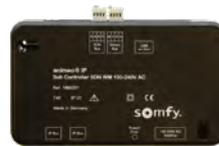
The IP Sub Controller expands animeo IP/io installations. An IP Building Controller is essential for integration of an IP Sub Controller. It provides dynamic solar management by directly controlling Somfy-motorized window coverings and climate information given by a real-time weather station.
