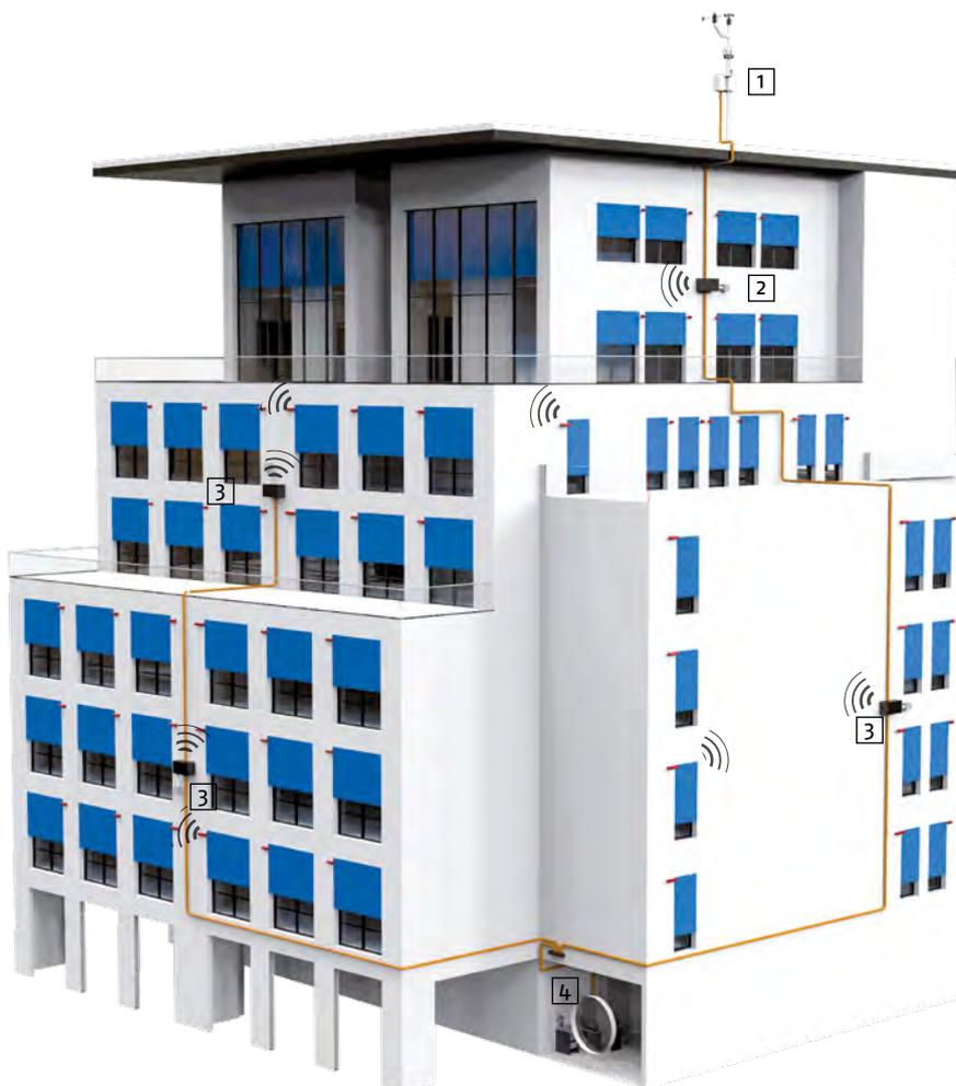
The animeo IP/io Building Controllers and Sub Controllers communicate bi-directionally with the motors through the USB/io Transceiver.
