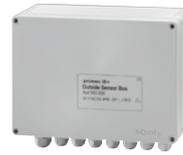
The Outside Sensor Box is the interface between the weather station, the Building Controller or Sub Controller. All measurement values are evaluated here and sent to the Building Controller. It requires an external 24 V AC/DC power supply.
