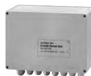
The Outside Sensor Box is the interface between external sensors and LON Sensor Interface. All measurement values are evaluated here and sent to the LON Sensor Interface. It requires an external 24 V AC/DC power supply.
