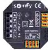
Motor Controller for motorized external Venetian blinds, roller shutters and windows. For the individual controlling of a 1 x 230 V AC motor via a unlocked serial push button and/or through Somfy solar shading management systems such as Somfy New Wired Range and Somfy animeo IB+. Available for flush mounting (IWM).
