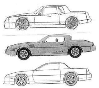
allowed. Stock size/height/length A and B pillars, no lowering or moving the full stock sized roof.
