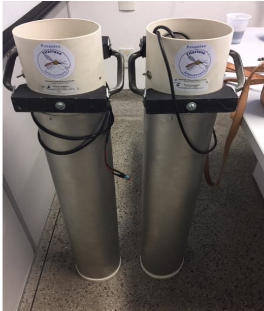
Mechanical vacuum aspirators
