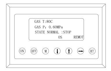
ON—start: press this button can start the motor
