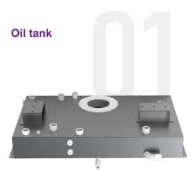
The oil tank is integrated with the cooling water tank, and the internal partition is designed to help the lubricating oil returning to the oil tank to better separate the air contained in it, avoid the oil pump cavitation, and reduce the liquid level fluctuation caused by the impact of the oil return.
