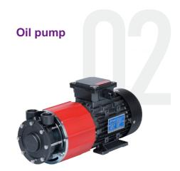
The magnetic pump, the pump body is made of stainless steel, can work in the medium -60°C to +350°C temperature range, low noise, small vibration, magnetic force driven between the pump body and the motor, the pump body has no dynamic sealing components, stable sealing performance, zero leakage.
