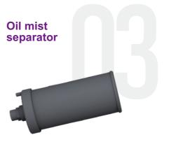
The oil mist separator is installed on the oil tank, so that the inside of the oil tank is communicated with the atmosphere, to ensure that the oil return is smooth, and to effectively intercept the overflowed oil mist from the oil tank, to prevent the oil mist from entering the box and being inhaled by the main engine and affecting the quality of the compressed air.
