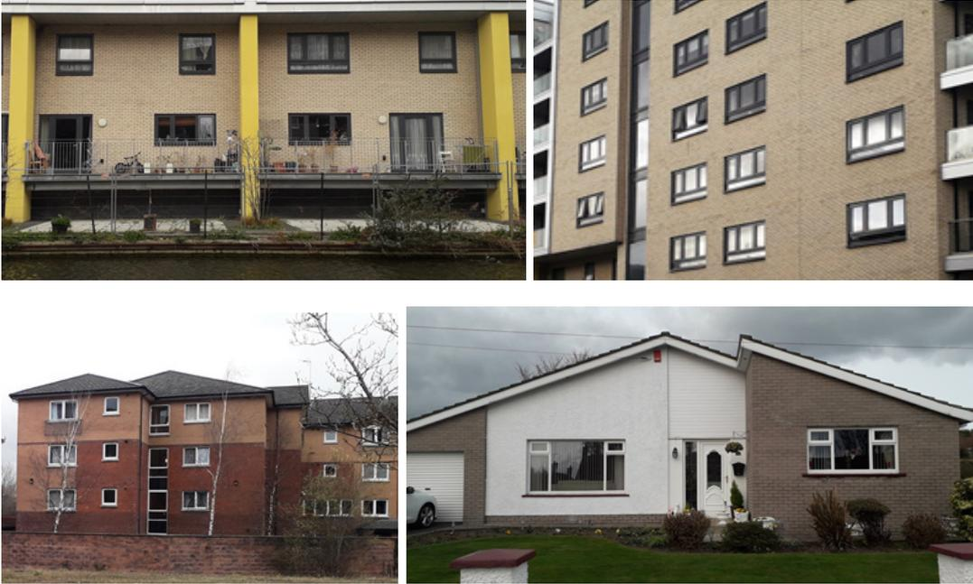
Figure #6-1: Examples of glazing proportion below 35% of facade area
