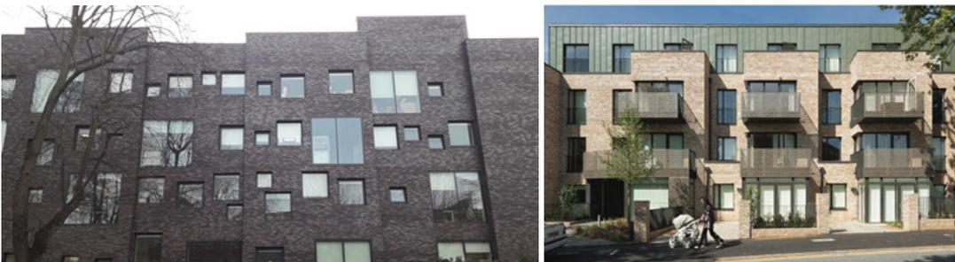
Figure #6-3: Examples of glazing proportion between 50 and 65% of facade area; (left) on upper end, un-mitigated; (right) Colby Lodge, with shading through balconies and articulation (Pollard Thomas Edwards)
