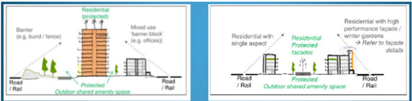
Figure #3-3: Examples of site layout mitigation measures.
