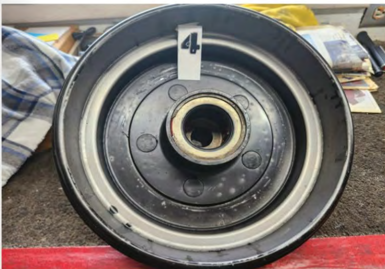
New brake drum with new grease seal and snap ring installed, ready to be put on the spindle.
