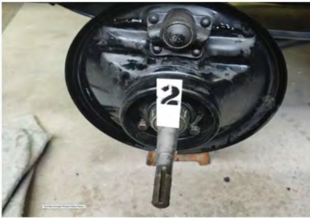
One of the front spindles and backing plates ready for new brake shoes.
