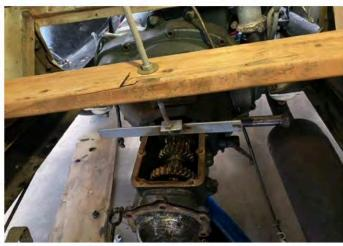
One shot you can see my rear heavy duty rubber engine mounts also, actually off a big helicopter, I added two lateral composite blocks to stop the engine moving laterally to reduce steering wander. If anyone's interested I can show closer detail and have two of the mounts spare.
