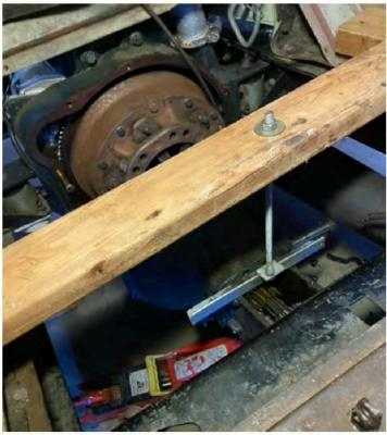
I fabricated two bits of 4 x 2 and laid one down either side of the chassis, chiseled out slots for the body mounting bolts. Then a length from side to side and drilled a hole in the center for the 10mm threaded rod. Drilled a piece of angle to bolt to the front top cover holes and a hole through the
