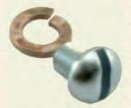
The problem is that the ignition cam screw may not hold the cam down tightly to the distributor shaft. After a bit of driving, the cam rotates into a more and more "retarded" position and the engine loses power.
