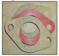
**Important Note:** You must use new / longer 1-inch bolts to compensate for the additional thickness. Failure to replace bolts will result in damaged carburetor flange threads and the carburetor will not be secure to the manifold.
