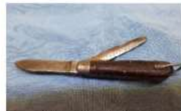
Figure 5 Utility knife with blunt blade
