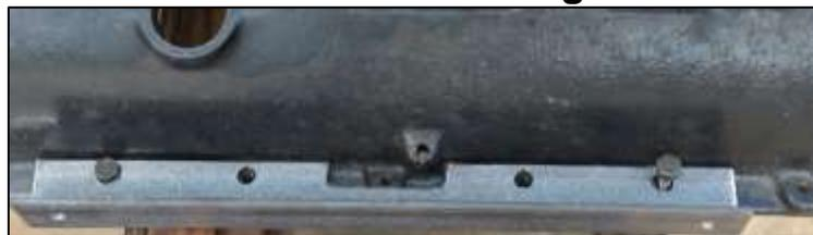
After fabrication, tack weld brackets A and B together, making sure that the flange spacing distance measures 2 ¾ in. If 2 in. angle iron is substituted for brackets A, B, and C, the flange distance needs to be adjusted to 3 ¼ in. Finish the assembly by applying a continuous fillet weld on both sides as shown in the assembly figure above.
