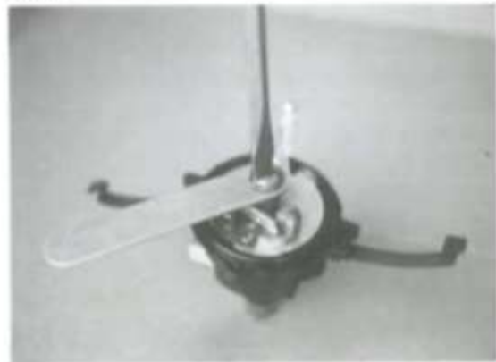
The cam is held in a precise position while tightening the cam screw.
