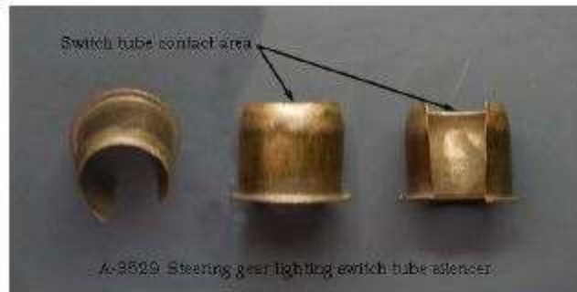
Three views showing the shape of the "silencer"
