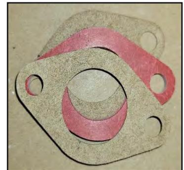
**Important Note:** You must use new / longer 1-inch bolts to compensate for the additional thickness. Failure to replace bolts will result in damaged carburetor flange threads and the carburetor will not be secure to the manifold.
