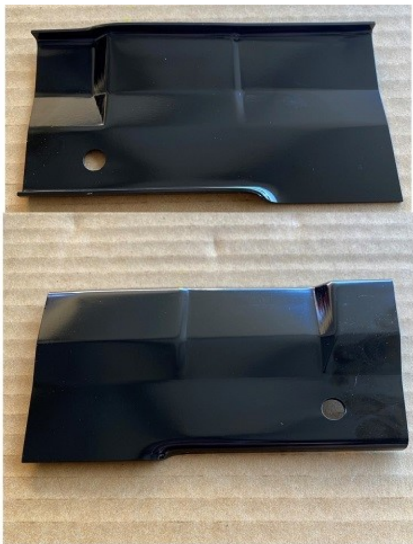
#207 XA-XC Upper Plenum Rect Reinforcing Plate LH
