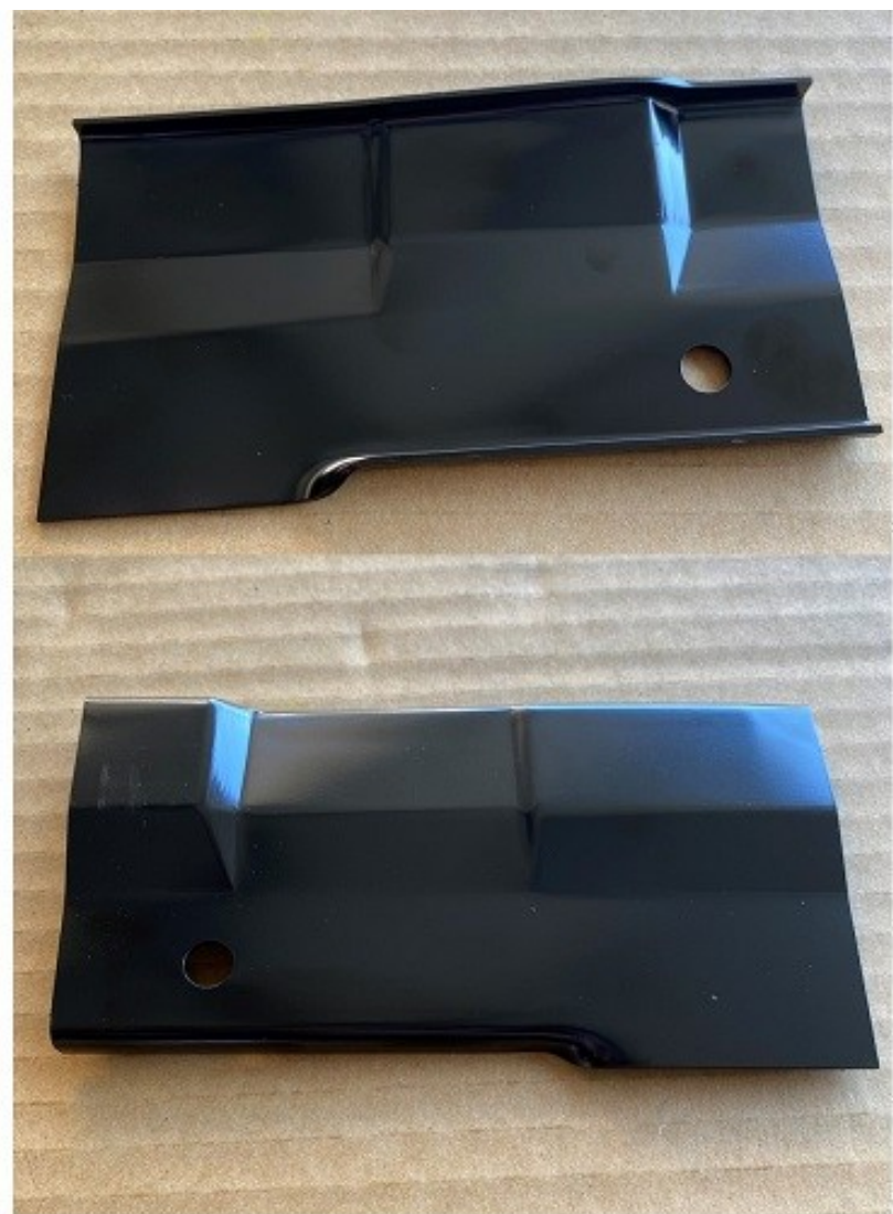
#208 XA-XC Upper Plenum Rect Reinforcing Plate RH
