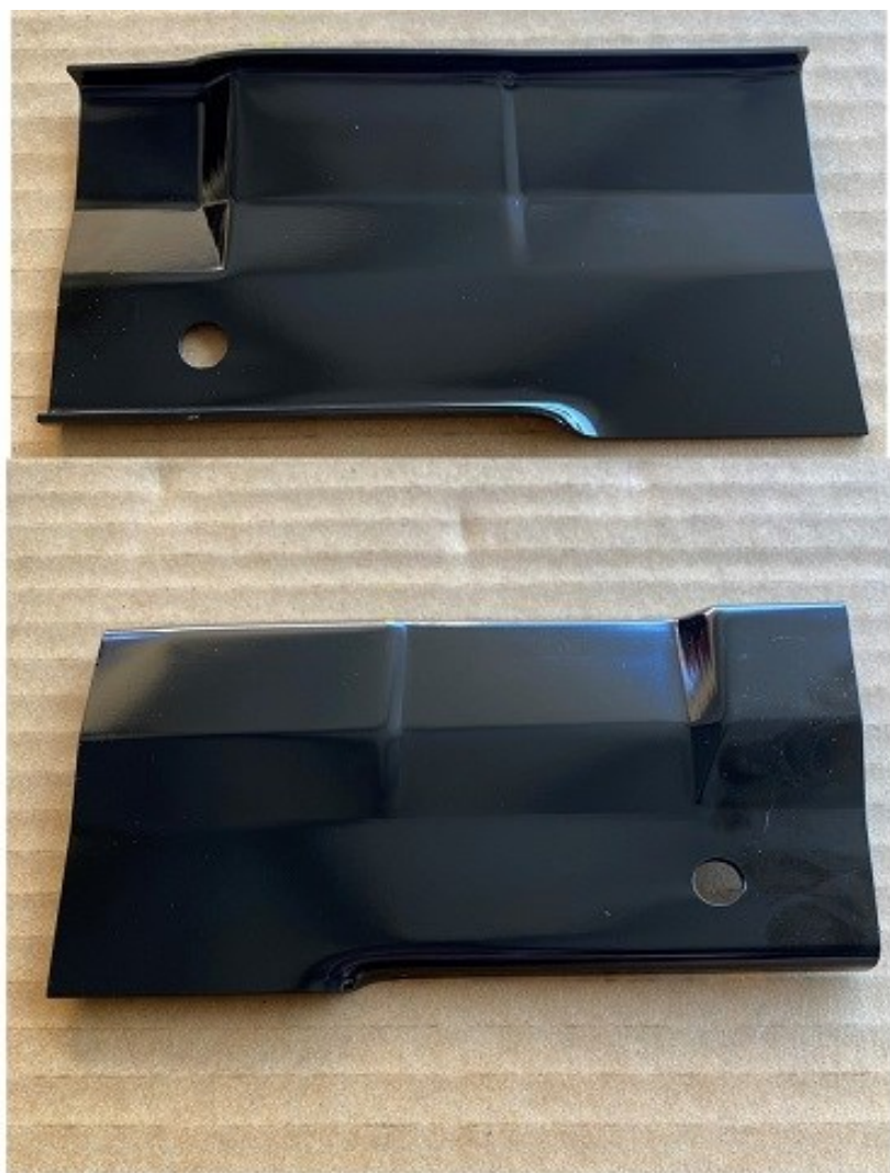
#207 XA-XC Upper Plenum Rect Reinforcing Plate LH
