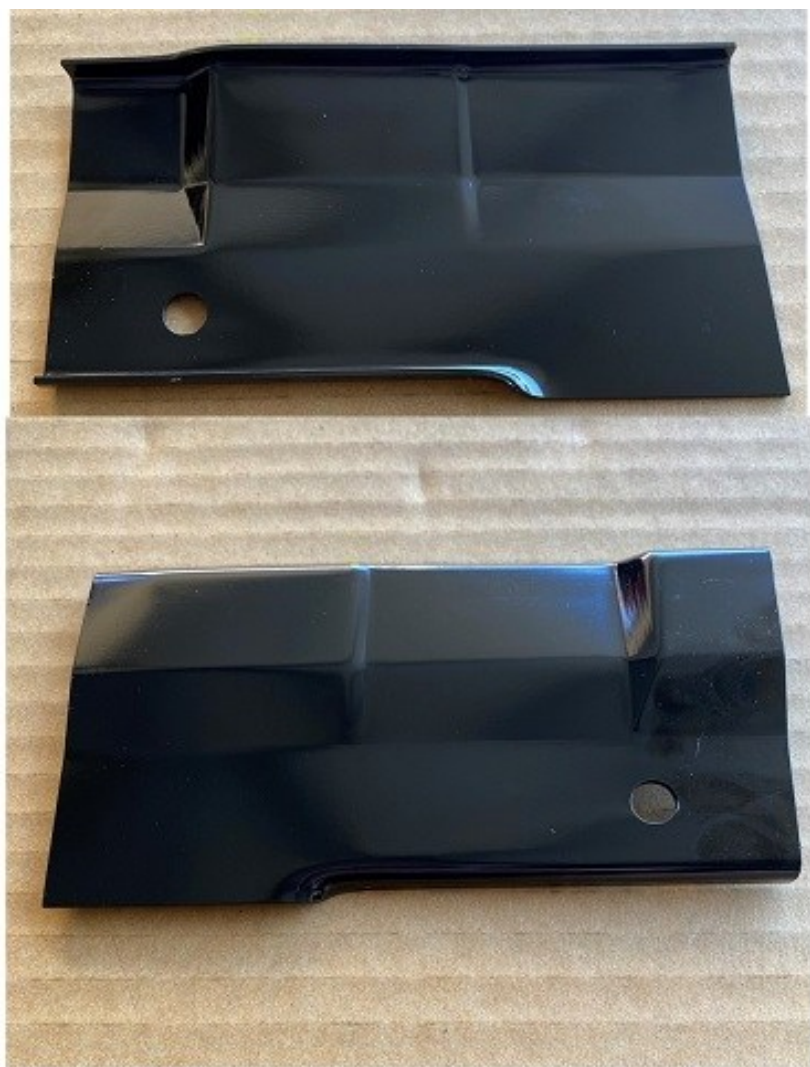
#207 XA-XC Upper Plenum Rect Reinforcing Plate LH
