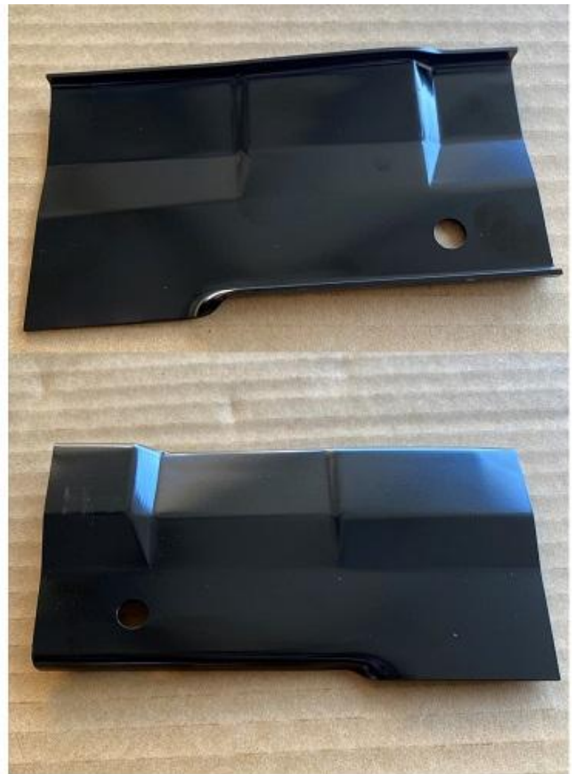
#208 XA-XC Upper Plenum Rect Reinforcing Plate RH
