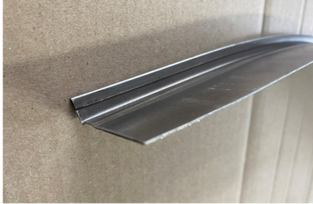
#232. XA-XC Sedan Gutter Repair LH
